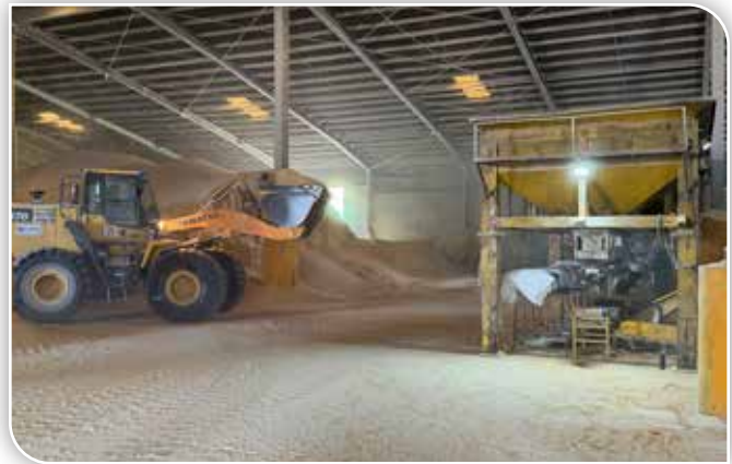
U.S. soymeal being moved by payloader into a bin for loading of 50kg bags for delivery to customers.
