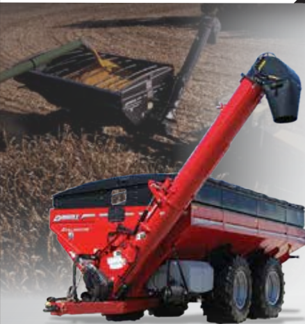
AVALANCHE DUAL-AUGER GRAIN CART FROM 2,500- TO 1,100- BUSHEL CAPACITIES
